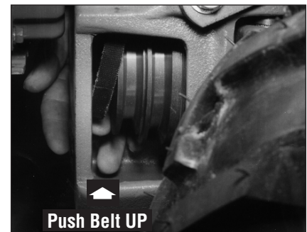
Figure 5-18: Push belt upward to create slack.
